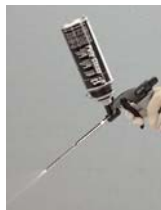
Attach can to gun basket to remove foam from gun barrel.
